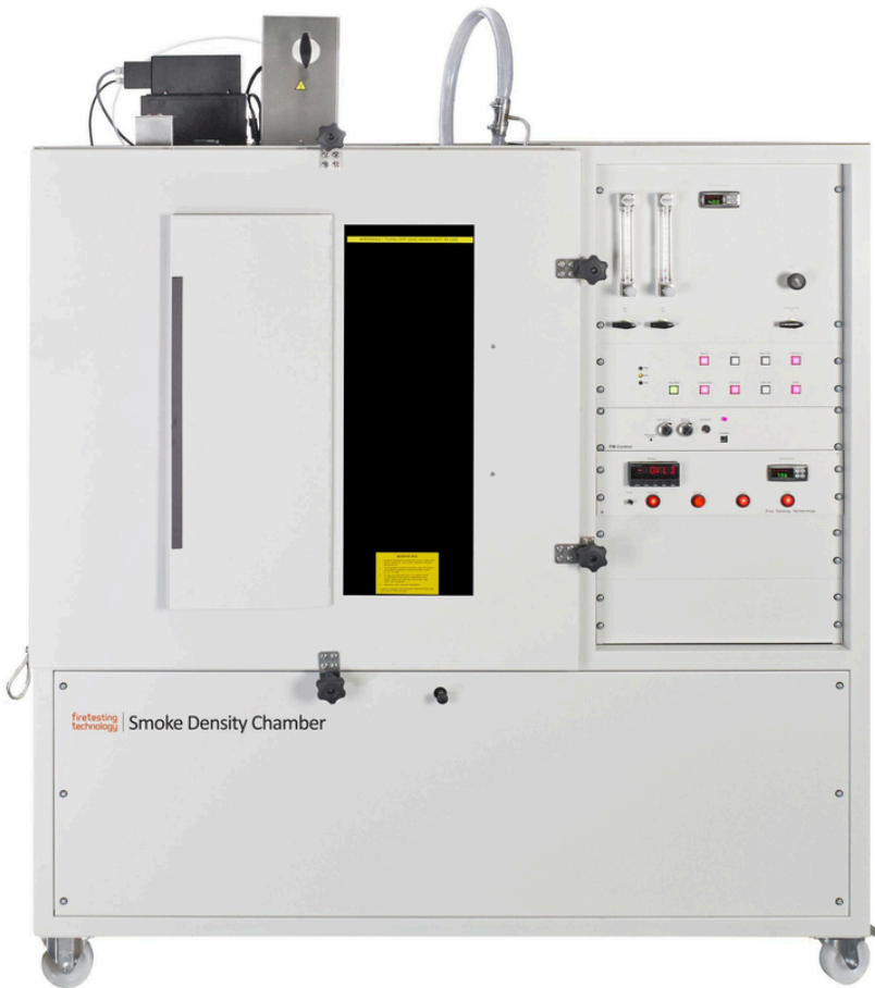
Fig. 2 : Smoke Density Test Chamber
