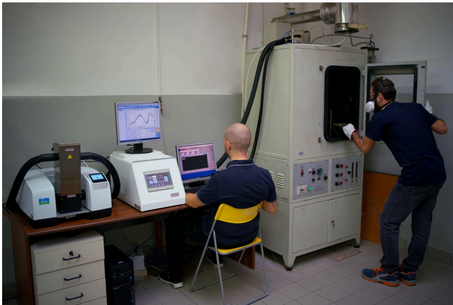
Fig 5 - ISO 5659 Smoke Density Test Setup
