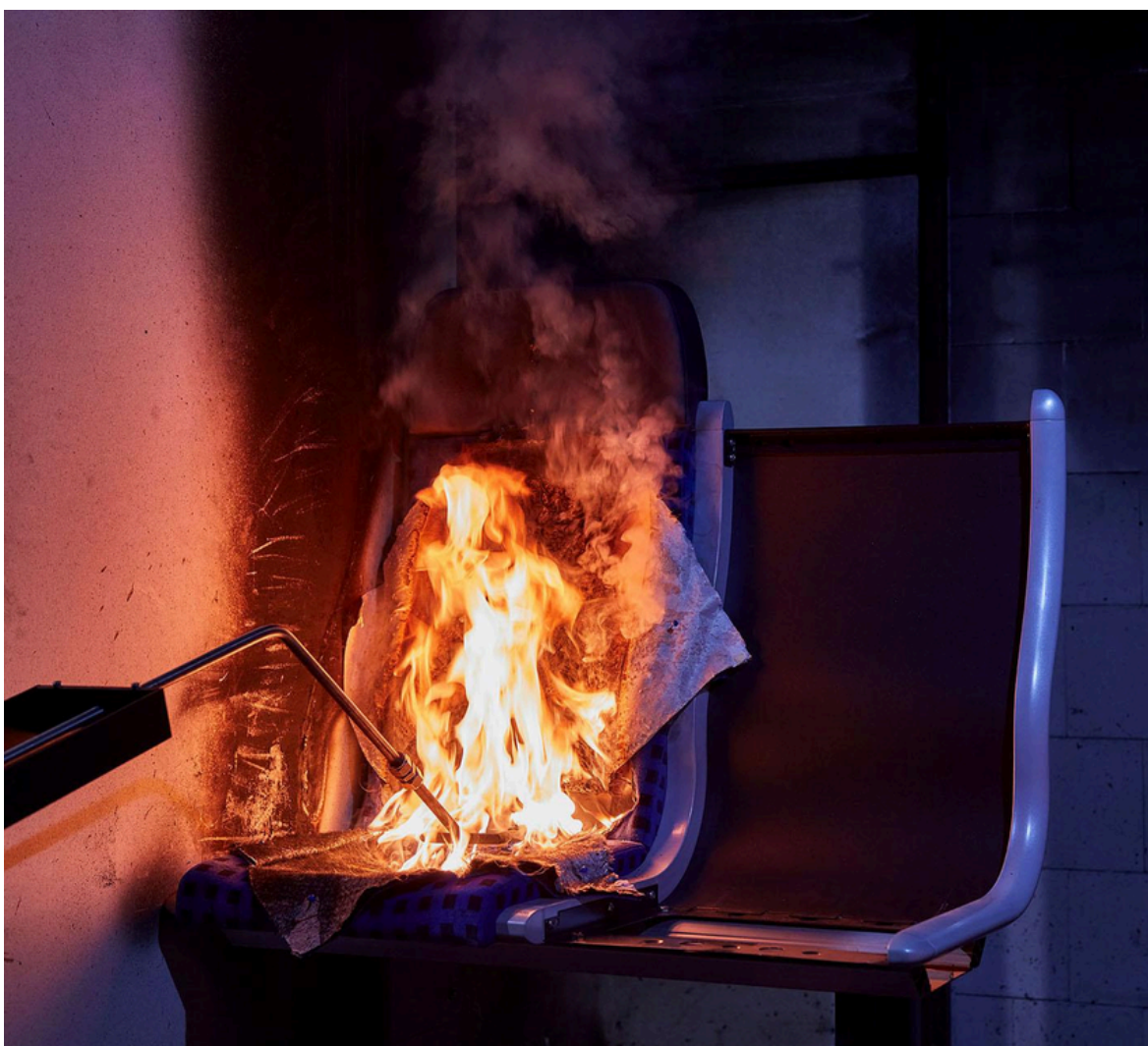
Fig 6 - Railway Seat Assembly Under Flame Spread Testing
