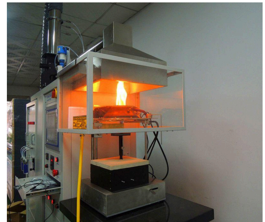
Fig 3 - Cone Calorimeter Testing Equipment
