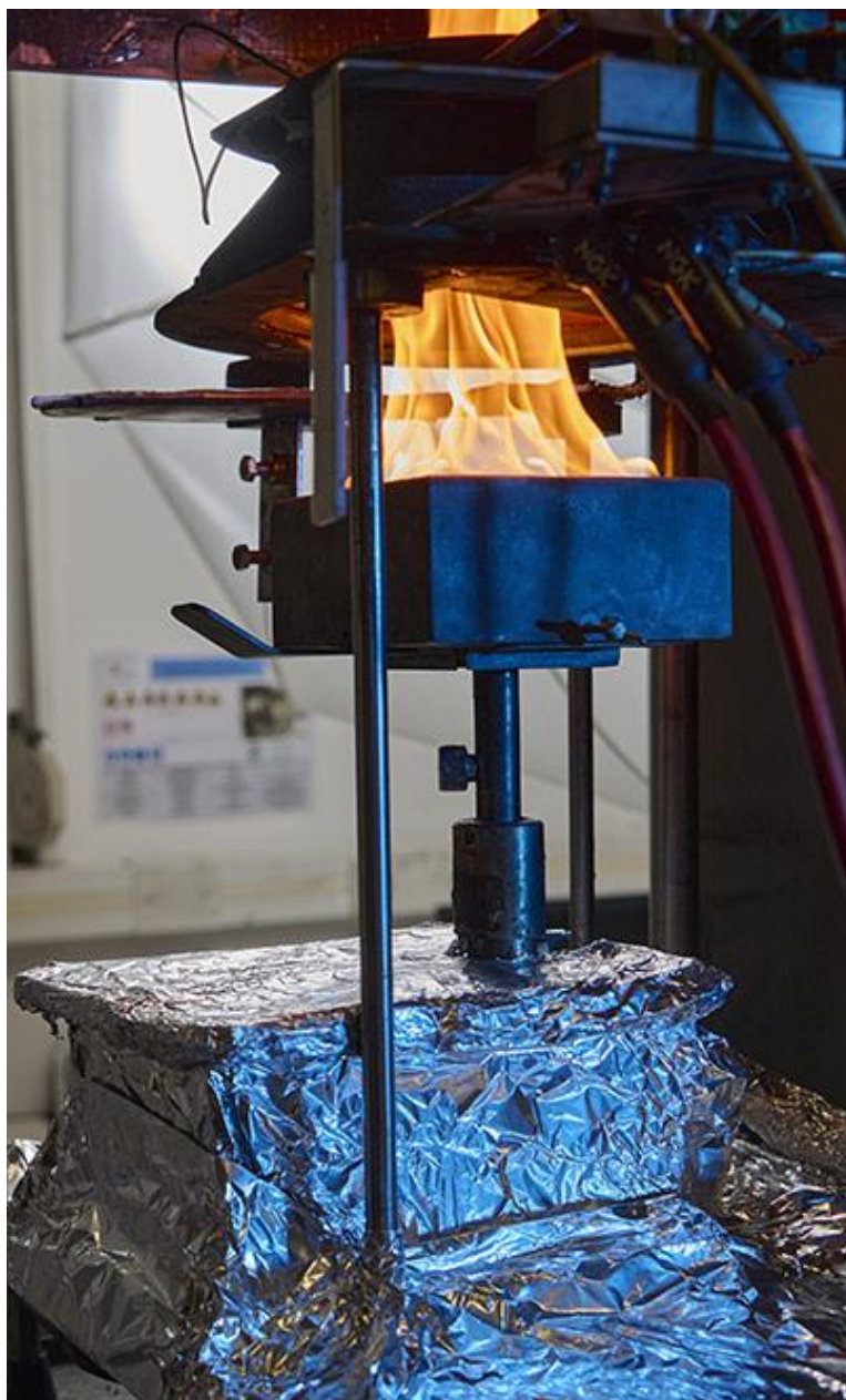
fig 3 : EN 45545-2 testing simulates fire conditions in railway environments to assess passenger safety risks.
